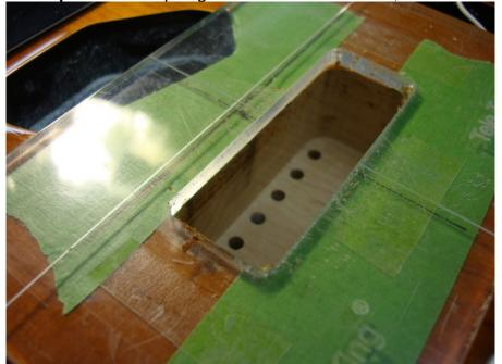
5. After using template as guide for initial rout, plunge as deep as the 3/4" bit will go.
