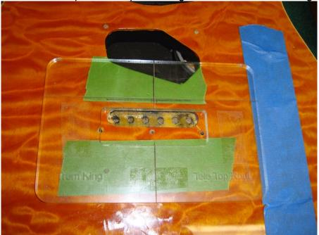
4. Cut Top Rout. Use plunge router with bit # 45491, 3/4" bit to start the rout.
