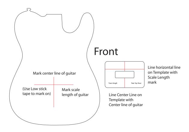
3. Locate Tele Top Rout template along centerline and scale length line on body.
